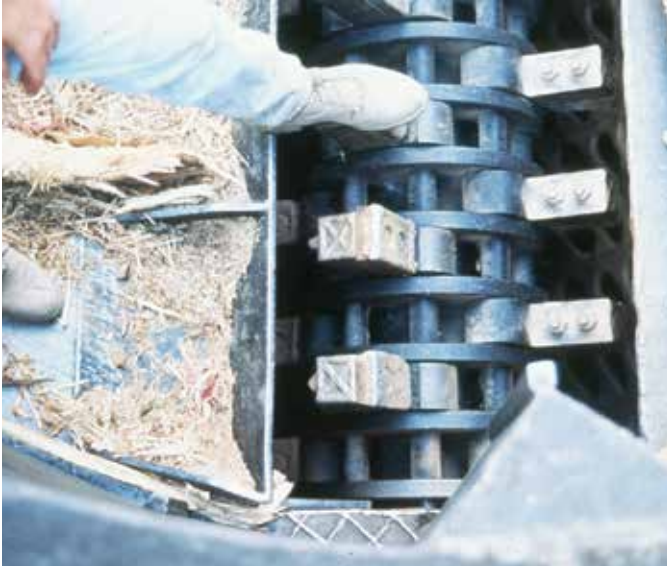
Tub grinder hammers for pulverizing into chips
