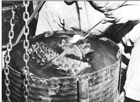
Built up tooth being sharpened by washing down Tube Borium "H" deposit with the flame.
