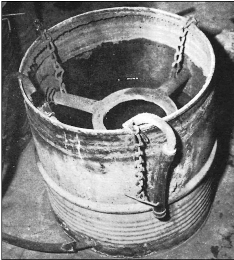
Fixture used for suspending bit at proper level in water while it is being welded.
