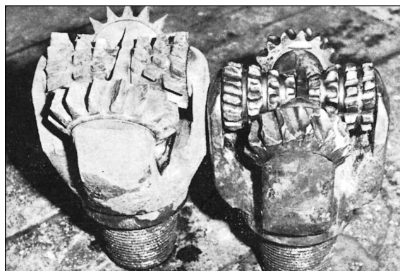
Rock bit on the left has been retipped with Stoodly Tube Borium "H". Bit on right is shown as worn.
