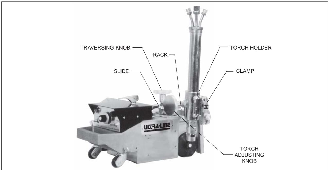
**Figure 2. Single Torch Rigging**
